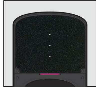
SIMPLESTOP DISMOUNT While performing a Simplestop™, Lightbar turns a steady magenta.
