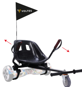
Turn right Pull up the right handle, push down the left handle.
